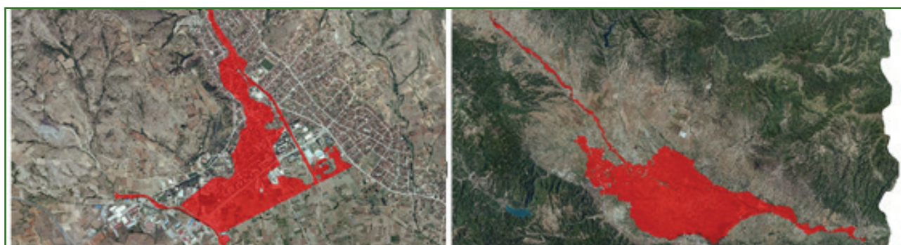
Figure 9 -Potential Q_{100} floods in Radovich city (by torrents Sushica and Radovichka Reka) and in the valley (by river Strumica)
